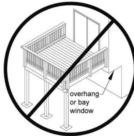
Figure 18. No Attachment to House Overhang with Ledger.
